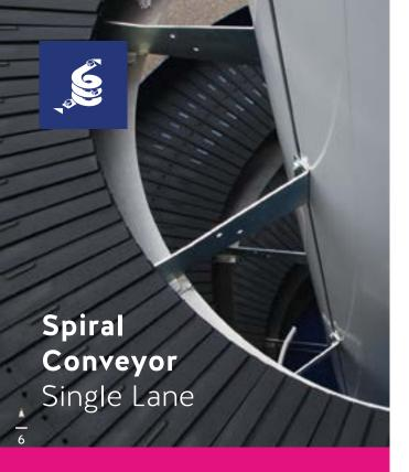
The APOLLO Spiral Conveyor is a proven reliable concept in vertical conveying, designed to conserve valuable floor space. The guide system includes low friction steel bearings and the chain is made of a heavy duty chrome plated steel construction. The guide rails are made of polyurethane embedded in an extruded aluminium profile. The slats are of moulded reinforced polycarbonate.
